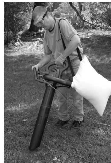
Figure 4-8: Picking up debris with vacuum
